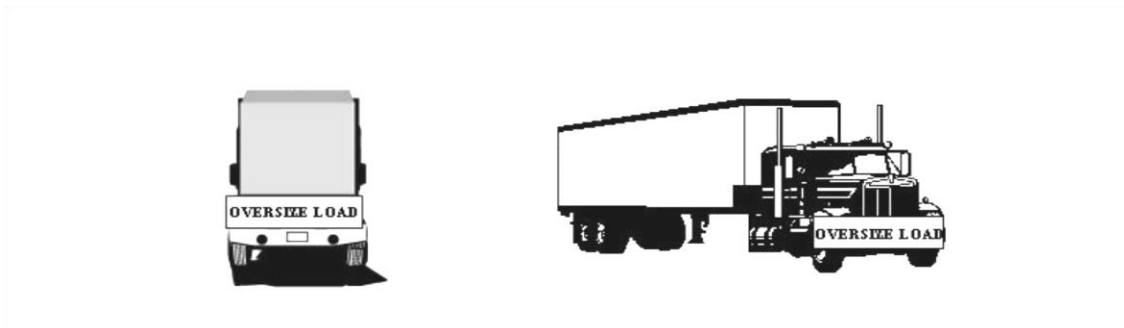
Warning Signs On Loads Over 10 Feet Wide
